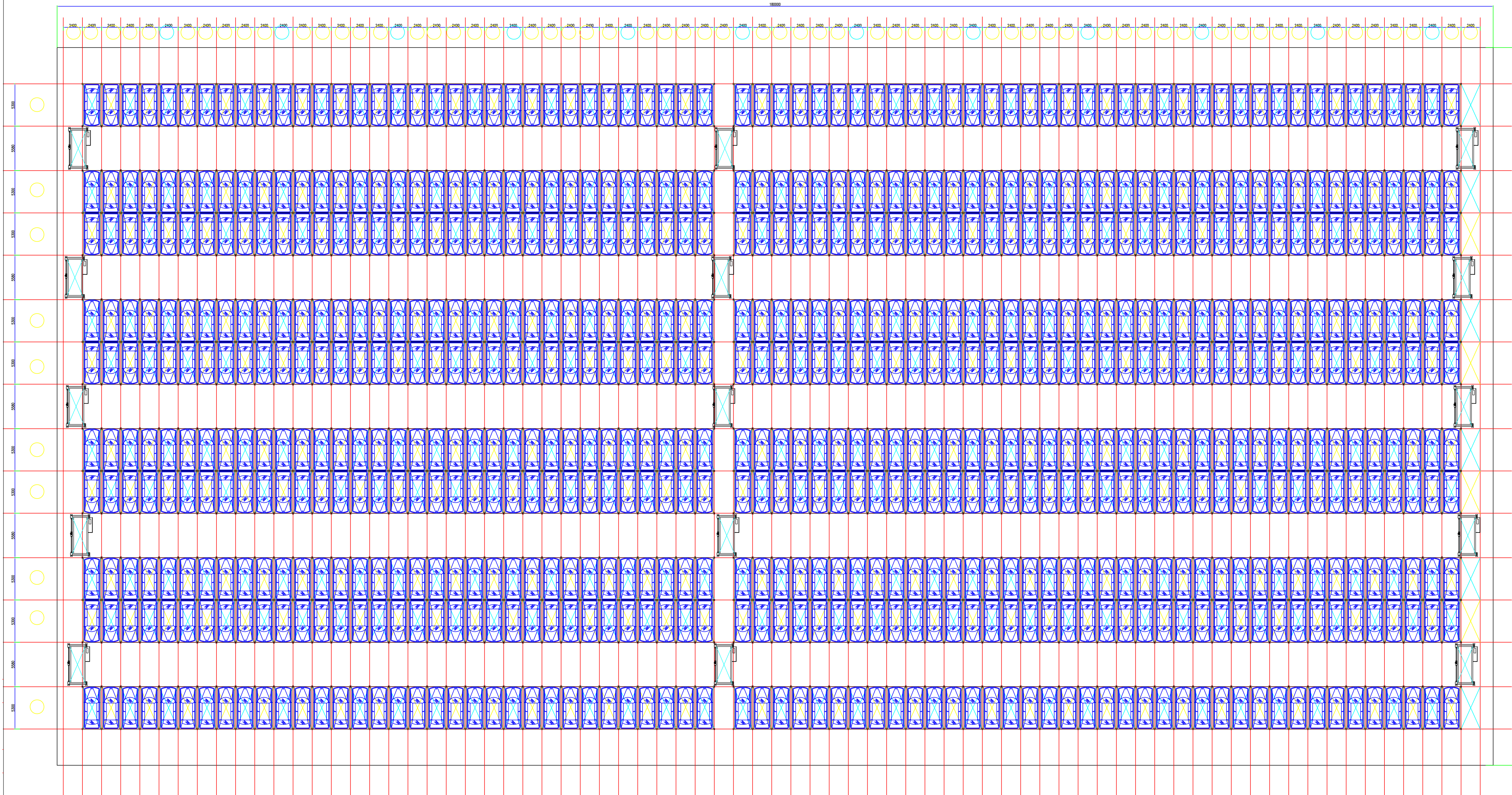
This plan can provide 240 car lots. The system used PPV parking system.
